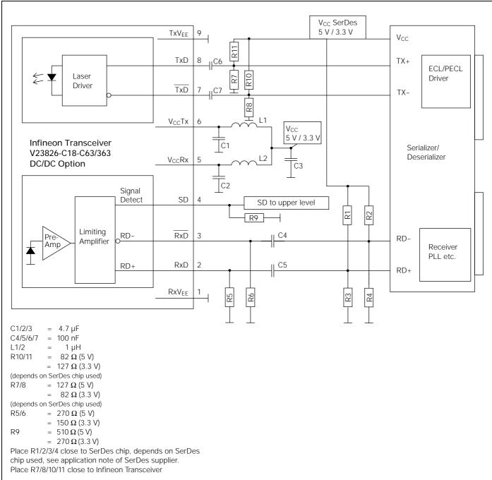
This Application Note assumes Fiber Optic Transceivers using 5 V power supply and SerDes Chips using 3.3 V power supply. It also assumes no self biasing at the receiver data inputs (RD+/RD-) of the SerDes chip (Refer to the manufacturer data sheet for other applications). 3.3 V-Transceivers can be directly connected to SerDes-Chips using standard PECL Termination network.
